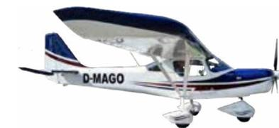
Sila 450C is a high-winged, single engine, two seated aircraft, with a semi-monocoque fuselage structure, made of approved aeronautical aluminum (6061 T6, 2017 T4, 2024T3). The wing airfoil is NACA 5417 and wings are rectangular with sweep a angle equal to zero.
