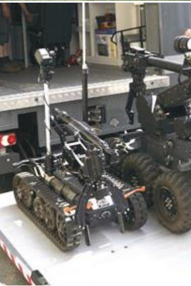
HBA RMI is equipped with a modernized PTZ (Pan Tilt Zoom) camera head, which allows to observe both the area around the robot and objects in the far distance (30x zoom). The head may be provided with one or two cameras, including an infrared unit. Owing to the use of Direct Drive type of motors , the cameras can perform both very fast and very precise movements.
